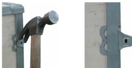
Figure 2-1 Straightening the hook
