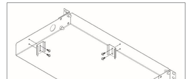
Figure 4.5 Attaching the Rails DIN to the Bracket of Vertiv™ MCR Kit High Temperature Alarm
