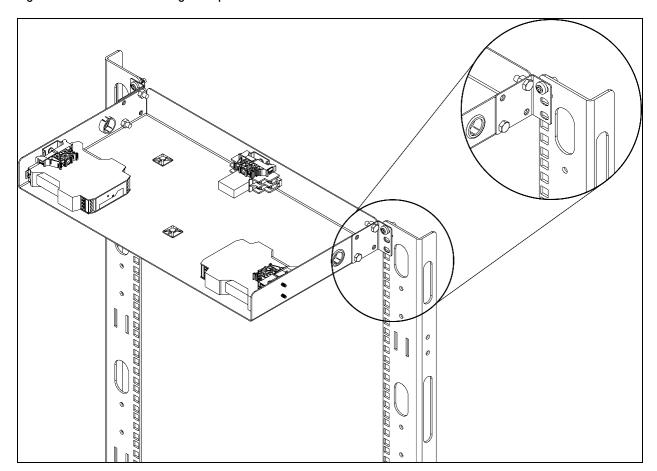
Figure 4.17 Vertiv™ MCR Kit High Temperature Alarm Bracket attached to Rails
