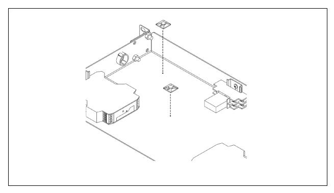
Figure 4.10 Attaching the Retainers to the Rail DIN
