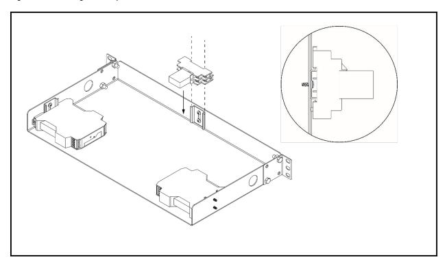
NOTE: The relay also must slide down through the DIN rail lugs until they contact the bracket of MCR Kit High Temperature Alarm. The relay should be fixed as shown in **Figure 4.7** above .
