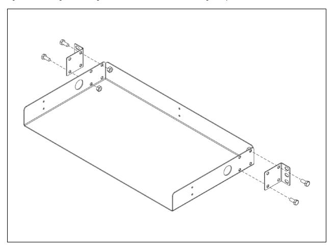
NOTE: Use the screw caps and the nuts hex to fix the components.
