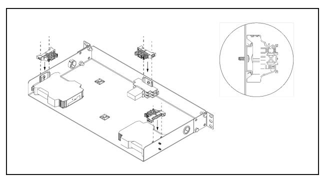
NOTE: In the same way as the converters and the relay, the retainers must slide down through the DIN rail lugs until they contact the converters and the relay. The retainers should be fixed as shown in **Figure 4.10** above .
