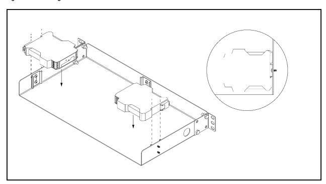
NOTE: The converters must slide down through the DIN rail lugs until they contact the bracket of Vertiv™ MCR Kit High Temperature Alarm. The converters should be fixed as shown in **Figure 4.6** on the previous page .
