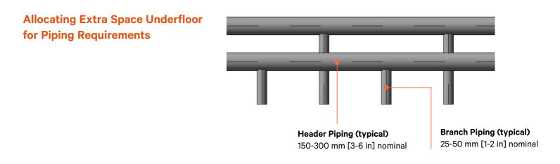
Underfloor designs for piping should leave adequate space for piping, insulation, and pipe crossover. Dimension will vary from site to site.
