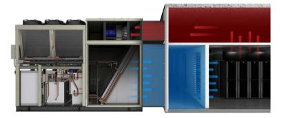
The Liebert DSE freecooling solution is scalable in 400kW and 500kW unit capacities, with both perimeter and rooftop configurations to support growing and changing data center loads and site requirements.
