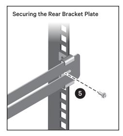
Tighten the screws to firmly secure the rear bracket plate to its rear bracket plate holder.
