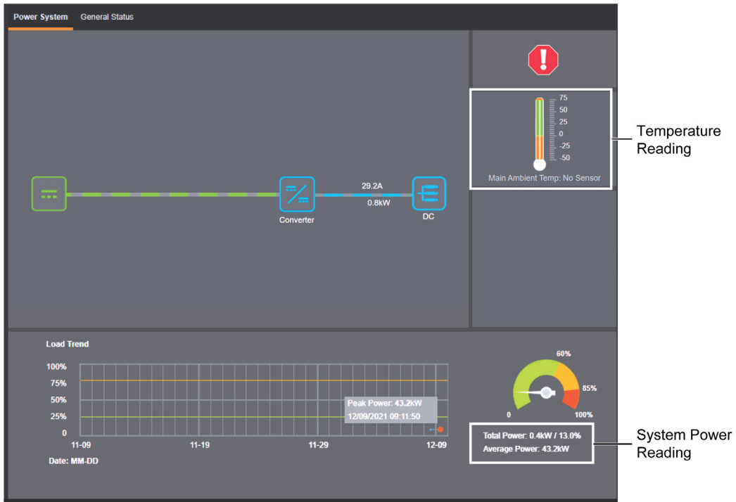
Figure 9-9 Power System Status Tab
