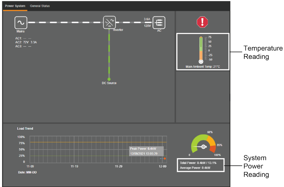
Figure 8-9 Power System Status Tab
