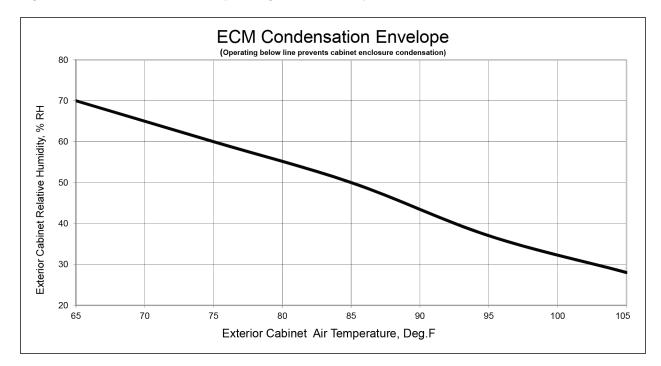
Figure 10.2 ECM recommended operating conditions to prevent excess cabinet condensation
