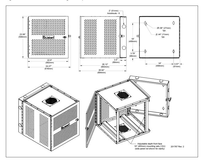
Figure 9.2 Liebert® MCR 12U hinged body wall-mount dimensions and features
