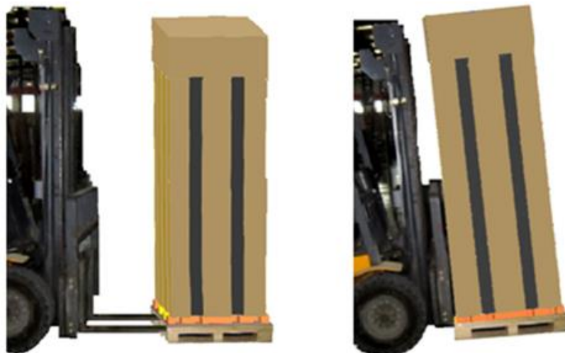
Figure 2-1 Moving the equipment using a Forklift truck
