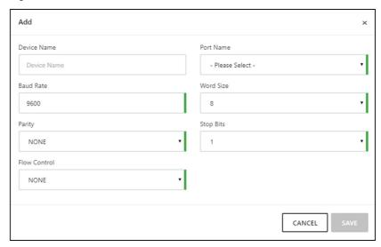
Figure 3-50 Add a console device
