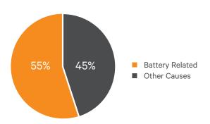
Figure 1: Battery-related failures account for more than half of all UPS system failures.
