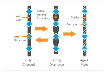
Figure 3: Batteries age when mechanical stress causes grid expansion.
