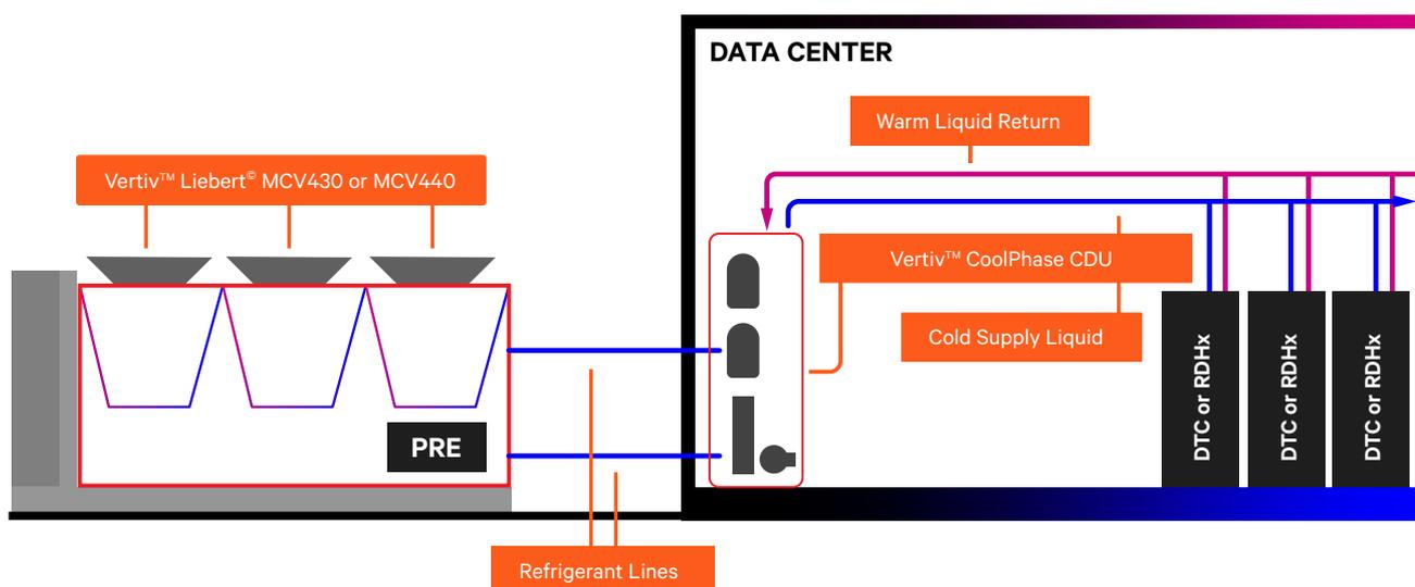
*Working in tandem with direct-to-chip cold plates or rear door heat exchangers, the Vertiv™ CoolPhase CDU utilizes pumped refrigerant economization (PRE) to eliminate the need for chilled water, allowing you to easily and efficiently cool pods of high-density racks in your air-cooled data center.*
