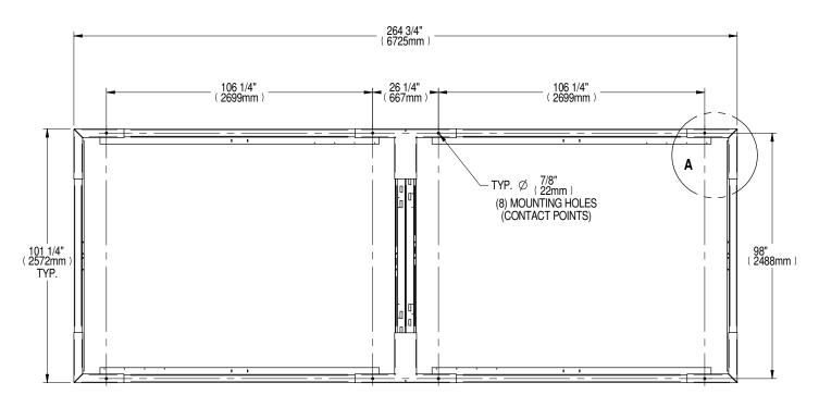
Underside of unit, coil and fan removed for clarity.
