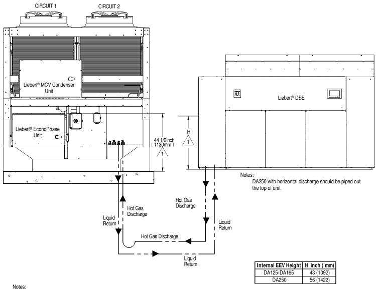
The outlet of the receiver must be higher than the elevation of the EEV inside the indoor unit.
