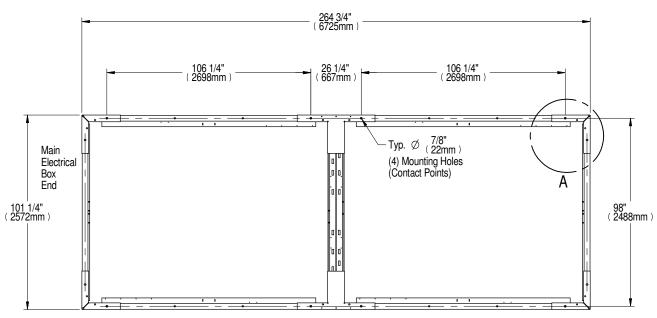
Underside of Unit Coil and Fans removed for clarity
