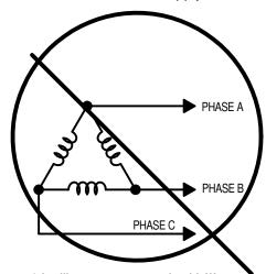
The 380-575volt unit is designed to operate with Wye-connected power with a solidly grounded neutral. It will not operate properly with Wye-connected power with high-resistance (or impedance) ground or with Delta-connected power. A separate neutral wire is not required to be run to the Liebert® MCV Condenser.
