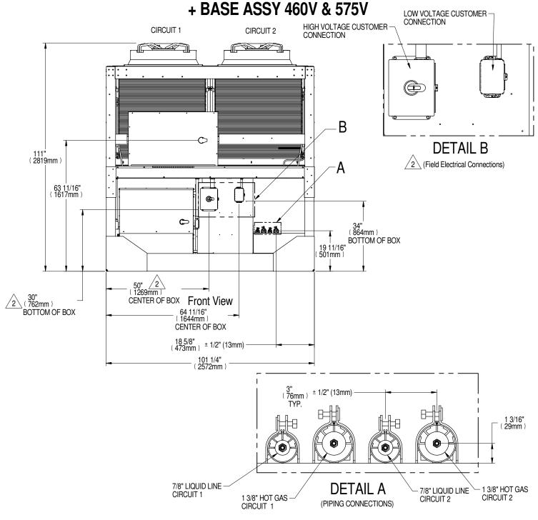
1. Field to provide hole for conduit for high voltage disconnect box and low voltage distribution panel.
