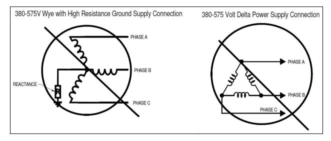
NOTE: The 380-575 volt unit is designed to operate with Wye-connected power with a solidly grounded neutral. It will not operate properly with Wye-connected power with high-resistance (or impedance) ground or with Delta-connected power. A separate neutral wire is not required to be run to the Liebert® MCV Condenser.
