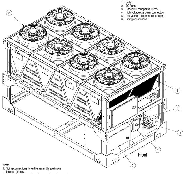
2. Electrical connections for entire assembly are located in high voltage customer connection boxes (item 4) and low voltage customer connection box (item 5).
