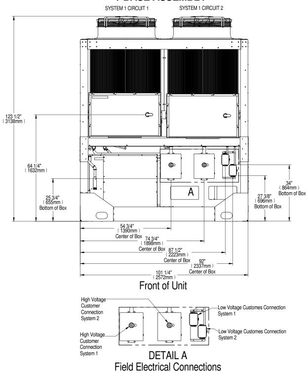
1. Field to provide hole for conduit for high voltage disconnect box and low voltage distribution panel.
