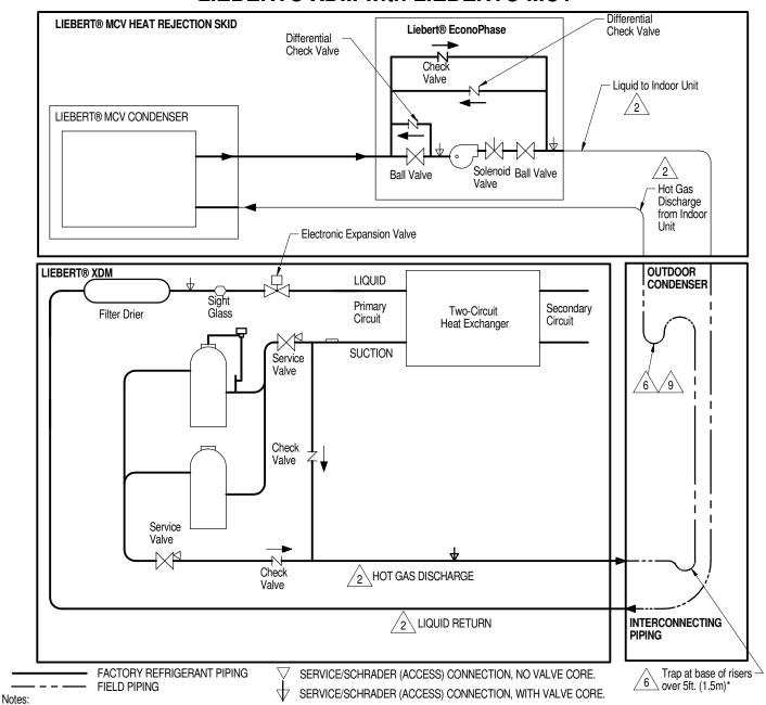
1. Two refrigeration circuits provided. Single refrigeration circuit shown for clarity.
