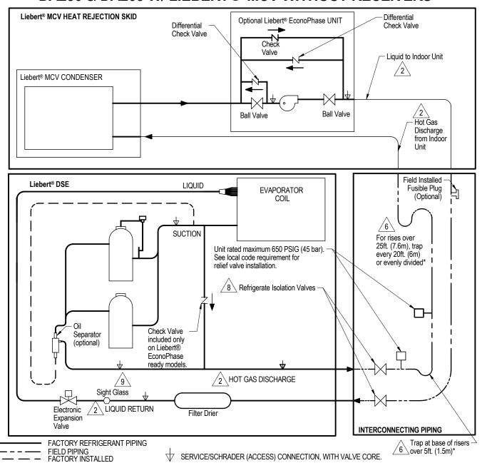
Notes Two refrigeration circuits provided. Single refrigeration circuit shown for clarity.
