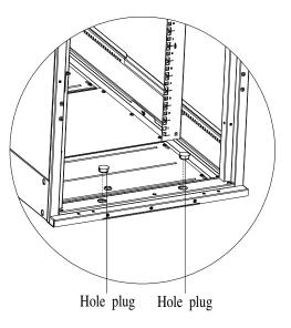
Figure 2-12 Hole Plug Head Mounting
