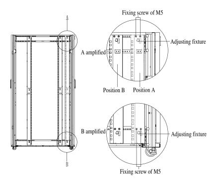
Figure 3-1 EIA Rail Adjustment
