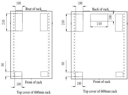
Figure 3-8 Top Cover Cabling Hole Size
