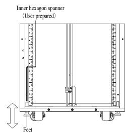
Figure 3-21 Adjusting Mode on Feet
