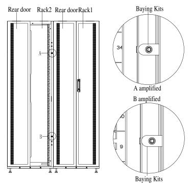
Figure 3-25 Baying the Rack in the Rear
