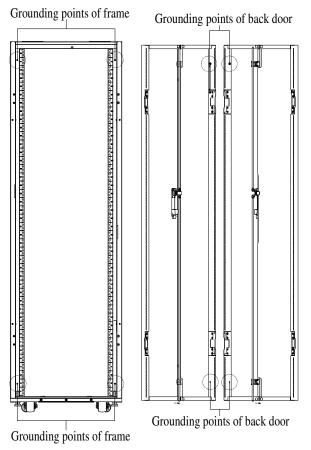
Figure 3-18 Grounding Points of Frame and Rear Door
