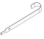
Figure 2-1 Floating Nut Hook
