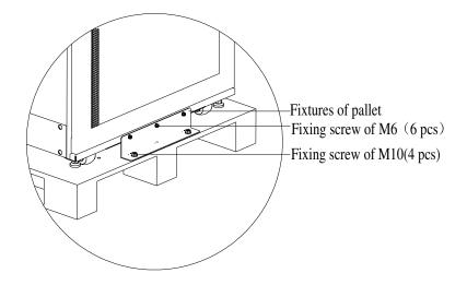
Figure 2-7 Disassembly of Pallet Fixtures
