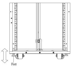
Figure 3-22 The Way to Adjust the Feet
