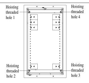
Figure 2-10 Rack Hoisting Hole
