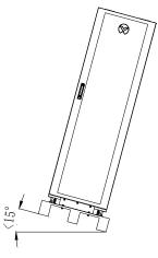
Figure 2-6 Maximum tilt angle on both sides of the rack (front view)
