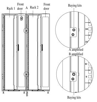
Figure 3-24 Baying the Rack in the Front
