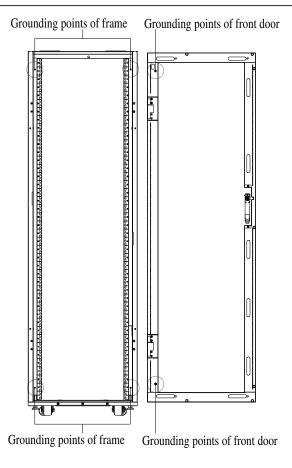
Figure 3-17 Grounding Points of Frame and Front Door
