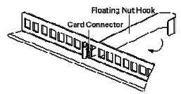
Figure 3-27 Floating Nut Mounting
