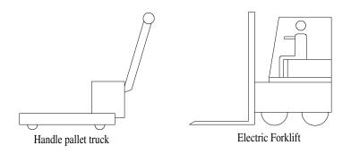
Figure 2-5 Mechanical Handling Tools
