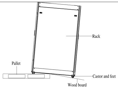
Figure 2-8 Removing the Pallet
