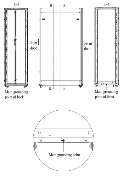
Figure 3-20 Rack Main Grounding Points
