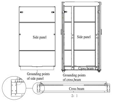
Figure 3-19 Rack Side Panel and Beam Grounding Points
