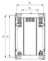
Figure 3-28 Position of installation hole at the bottom of the rack
