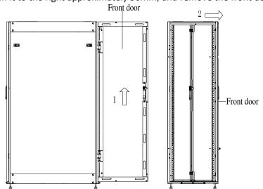
Figure 3-13 Remove the Front Door Schematic (Front Door Open)
