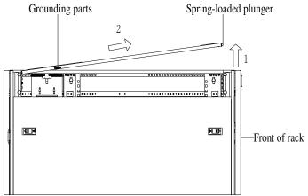
Figure 3-10 Disassembly of Top Cover
