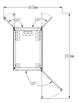
Figure 2-13 Space required to open the front and rear door of the rack (overlooking, unit: mm)
