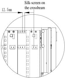
Figure 3-2 Diagram of Crossbeam Silkscreen
