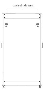
Figure 3-4 Side Panel Disassembly
