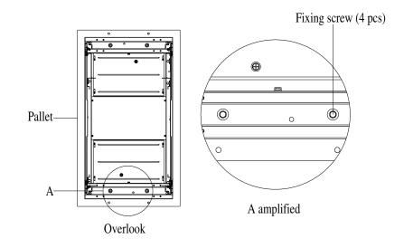
Figure 2-9 Pallet Disassembly Diagram
