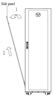
Figure 3-5 Side Panel Disassembly
