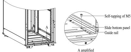
Figure 3-12 Bottom Panel Adjustment
