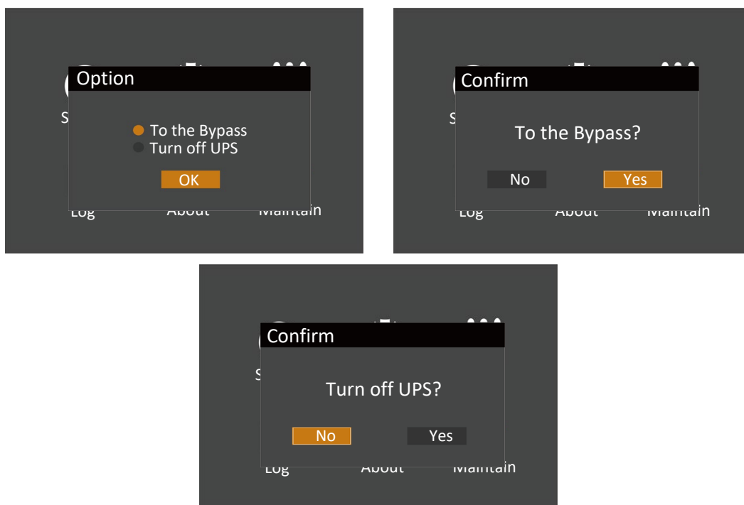
Figure 3-6 Bypass normal interface
